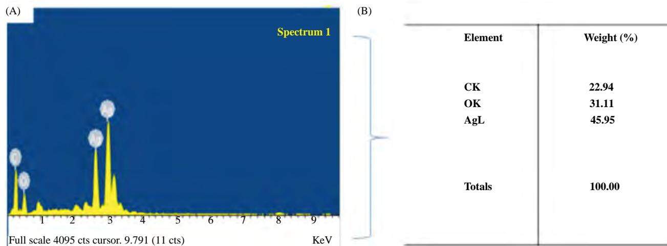
**Figure 4.** EDX investigation of AgNPs. A: EDX spectrum of AgNPs; B: Calculated percent elemental analyses.
